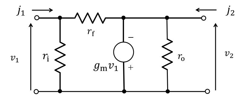
Obtain the Y matrix for the above equivalent circuit ( $\pi$ -shape circuit).
